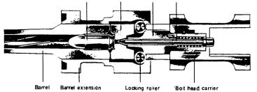
Ill.# 47A - Bolt group in locked (closed) position, ready for firing
